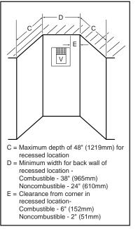
Figure 18 - Minimum Clearances for Vent Terminations
